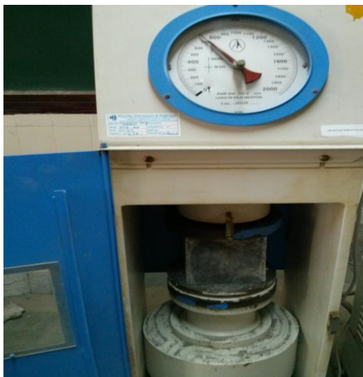
Fig 6.1 Compression testing of samples
