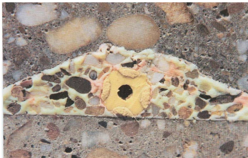
Figure 6 Reinjection of a honey-comb by duroseal inject (yellow: injection, red: re-injection) (Courtesy of Greenstreak Group, Inc)
