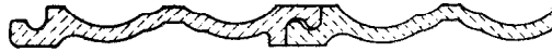
2B ARRANGEMENT OF THREE TILES BREADTHWISE IN TIGHT POSITION FIG. 2 MEASUREMENT OF TOLERANCES
